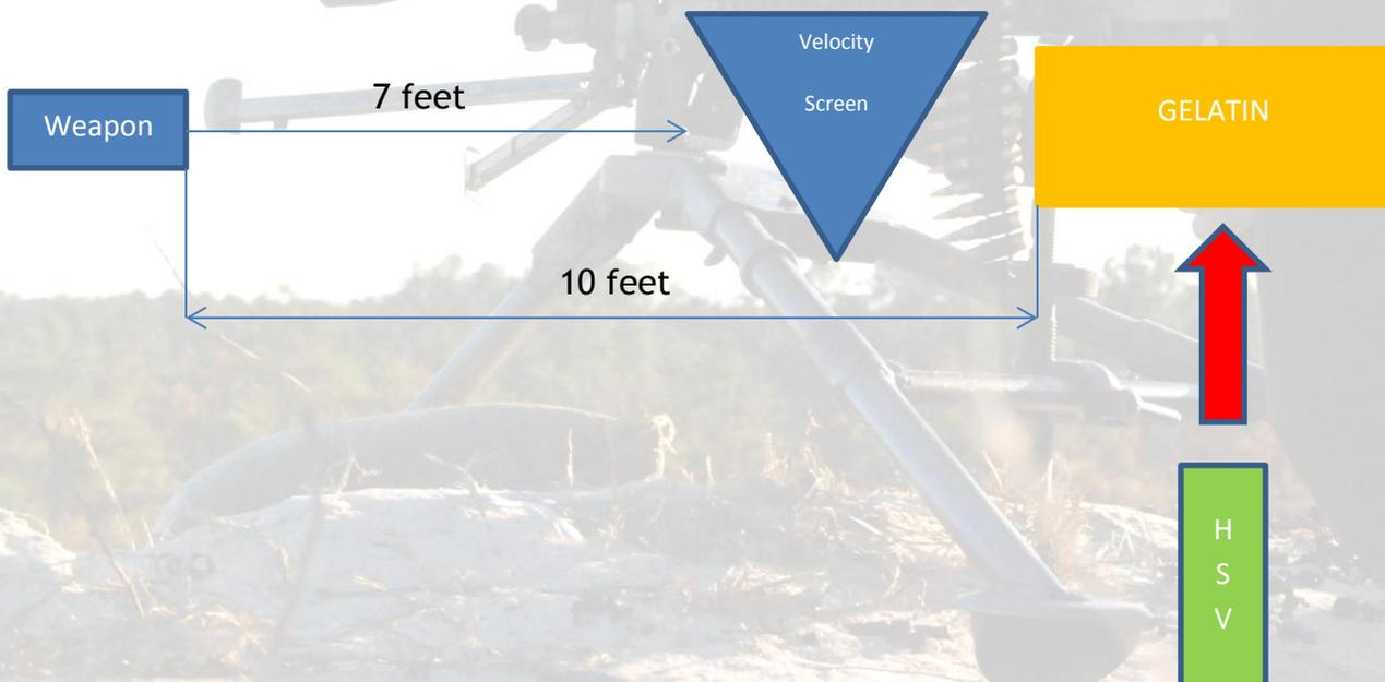
With the ultra slow motion camera in use being the Photron SA-5 Color. Atmospheric conditions at the test site were 76° F and 80% relative humidity and took place on 04 April 2014.
